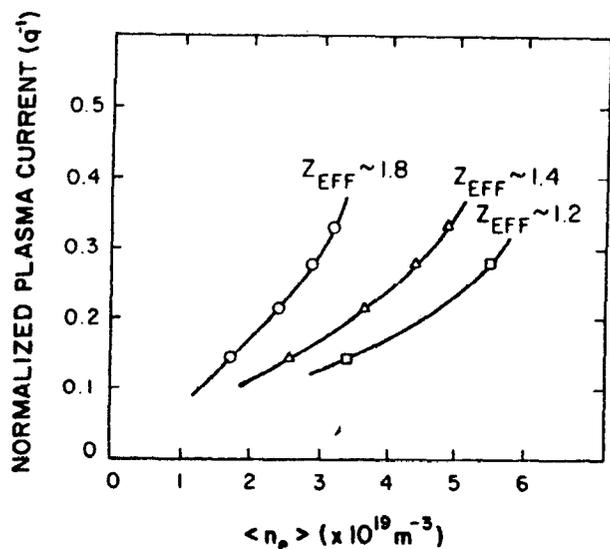
Figure 8: Maximum plasma density achievable at a given plasma current is dependent on impurity level. For pure DT plasma  $Z_{eff} = 0$ . Calculated result for JT60. Hirayama T, et al. J Nucl Mater 1986.
