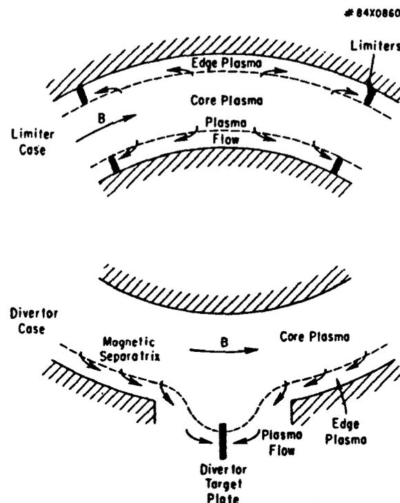
Figure 9: Schematic of limiter and divertor geometry. PMI at divertor target is located further from main plasma than for limiter target.
